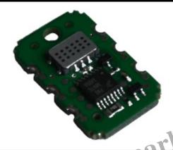
The <u>MiCS-VZ-89TE</u> combines state-of-the-art MOS sensor technology with intelligent detection algorithms to monitor tVOCs and CO2 equivalent variations in confined spaces, e.g. meeting rooms or vehicle cabins. The dual signal output canbe used to control ventilation on-demand, saving energy and reducing cost-of ownership.
